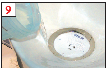
9 With diverter shield removed, fill cartridge with 1 quart or more of clean water until there are no air bubbles
